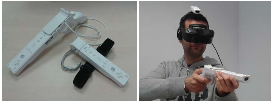
Fig. 4. Wiimotes with Motion Plus extension (left), and prototype in use (right)
